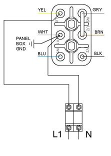
Figure 29: BE Generator Windings Schematic Diagram & AC Terminal Connections (16.0-23.0 MEG)
