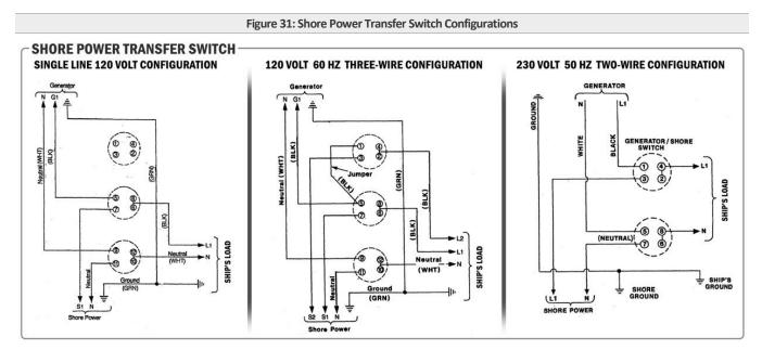
The second configuration shows connections for a two-wire 120-volt system from the generator with a threewire 120-volt boat system. In the second and third configurations, notice the repositioning of the white wire ground load on the terminal block to the generator case. No 240-volt equipment is permitted in the ship's load for the first and second configurations.
